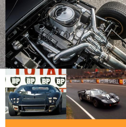
**Top Speed 205 MPH** 1964-1969 **Production** 7.0 liter 427 FE V8 Engine **Natural Aspiration** Valvetrain 2 Valves per Cyl, Pushrod **Fuel Feed** Holley 780CFM 4-Barrel **Displacement** 427.0 in<sup>3</sup> 485 bhp @ 6200 rpm **Power Specific Output** 69.32 bhp per liter **Transmission** 4-speed or 5-speed manual Drivetrain RWD w/LSD **Curb Weight** 2450 lbs 163.0 in Length Width 70.5 in Height 40.5 in 95.0 in Wheelbase
